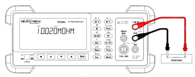
Note: Source current flows from the  $V\Omega \rightarrow to$  COM terminals Figure 3-3 Resistance Measurements
