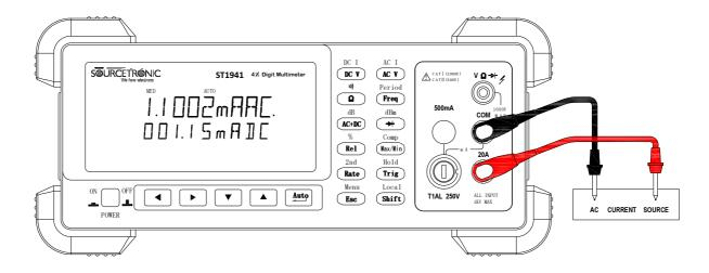
AC Current measurement on Range: 2A, 20A
