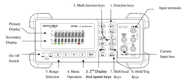
Figure 2-1 ST1941 Front Panel
