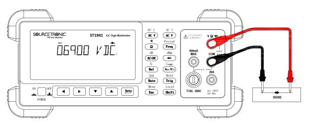
Note: Source current flows from the  $V\Omega \rightarrow to$  COM terminals Figure 3-6 Diode Measurement
