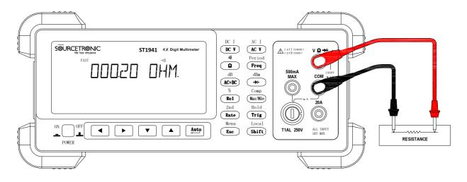
Note: Source current flows from the  $V\Omega \rightarrow to$  COM terminals.
